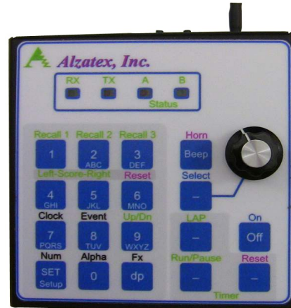
KP219A-RF2 wireless keypad with 18 buttons and a knob.
